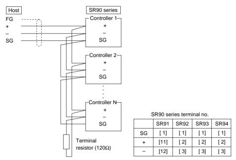
Note 1: In the case of RS-485, provide it with the attached terminal resistor of 1/2W, 120Ω across terminals + and if necessary. Nevertheless, it should be provided to only the last controller. If two or more controllers are provided with terminal resistors, correct operation cannot be guaranteed.
